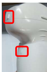
Make sure marker on the sensor holder is aligned with the probe
