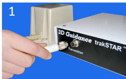
1 Connect magnetic generator to fusion controller
