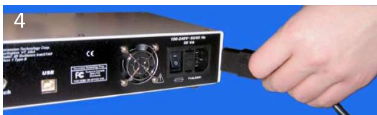
4 Power cable to fusion controller
