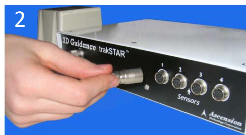
2 Connect probe sensor to fusion controller
